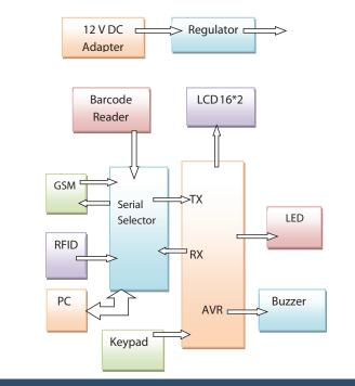
**Figure 1:** Block Diagram. Image source: Designed by Author.
