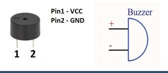
Figure 7: Buzzer & Its Pinout. Image source: Non-copyrighted Google Image.
