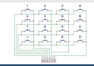
Figure 5: 4\*4 Keypad Matrix. Image source: Non-copyrighted Google Image.
