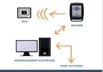
Figure 10: Process of RFID. Image source: Non-copyrighted Google Image.
