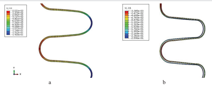
Figure 10: Displacement in the spring back a) with tie b) with friction.
