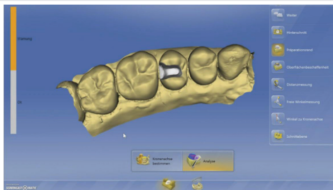
Figure 1: In the first step (1st Part), a first view is taken of the model to be assessed as an overview when the prepCheck is set to 'zoom to cavity' for approx. 1 second (Translation for: weiter = further, Hinterschnitt = undercut, Präparationsrand = preparation edge, Oberflächenbeschaffenheit = surface consistency, Distanzmessung = measurement of distance, freie Winkelmessung = free angle measurement, Winkel zur Kronenachse = angle of the crown axis, Schnitt Ebene = cut level, Kronenachse bestimmen = determine crown axis, Analyse = analysis, Warnung = warning).
