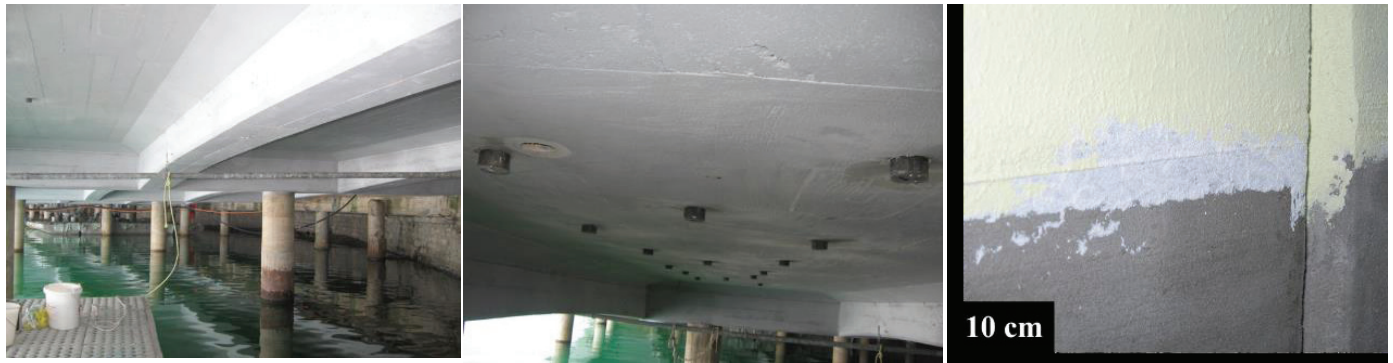
Figure 8: Multi-layer adhesion strength on a bridge (left), pull-off metallic cylinders with 50 mm diameter (center), and organic coating applied on several layers on the surface restored with mortar (right).
