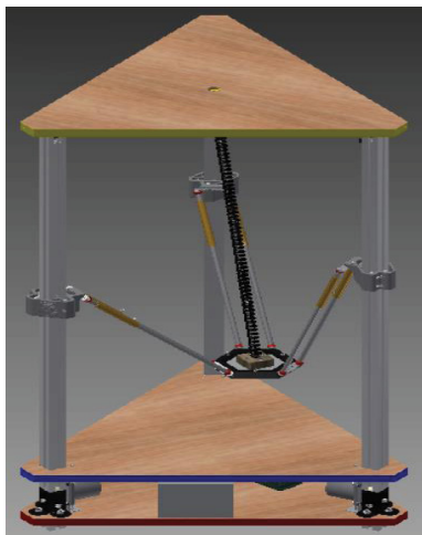
Figure 12: 3D CAD representation of the prototype. The whole assembly of the robot is present in this CAD file. Some of the noticeable elements are the prismatic joint modules, the fixed base of the robot, the parallelograms, the platform and the power supply and an eventual cable that goes from the roof of the robot to its end-effector platform.
