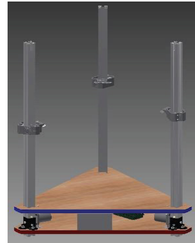
Figure 11: 3D CAD representation of the 3 prismatic joints modules already fixed to the base of the parallel robot. As it can be seen, each module is principally composed by an aluminium profile, a motor and the prismatic joint traveling along the column.
