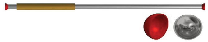
Figure 10: 3D CAD representation of the links used in the prototype and the detail of the spherical joints. The link length is adjustable by using a screw to fix an internal bar (silver) relative to the external one (copper).
