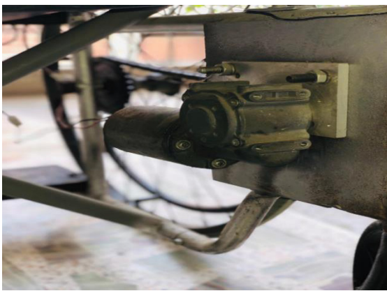
Figure 6: Motor coupled with gear box.
