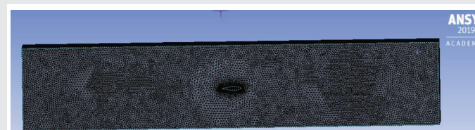
Figure 15: Wind tunnel mesh for back curved winglet 60°.
