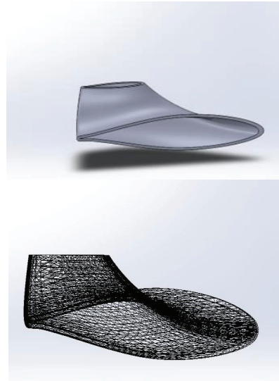
Figure 23: Winglet cad model and STL file for 3D printing.
