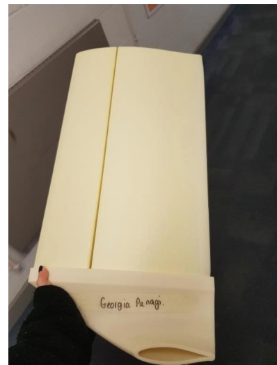
Figure 33: Wing and winglet assembly.
