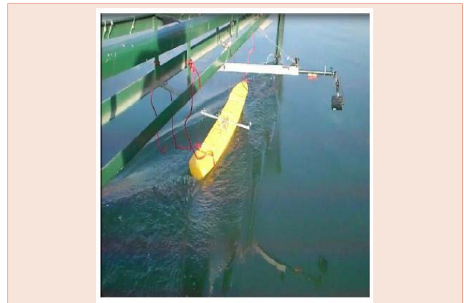
Figure 8: Model of container ship at time of testing.
